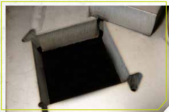
2 3/8 in. (60 mm) cut with WMS (using N 2 plasma and water secondary) at 800 A
